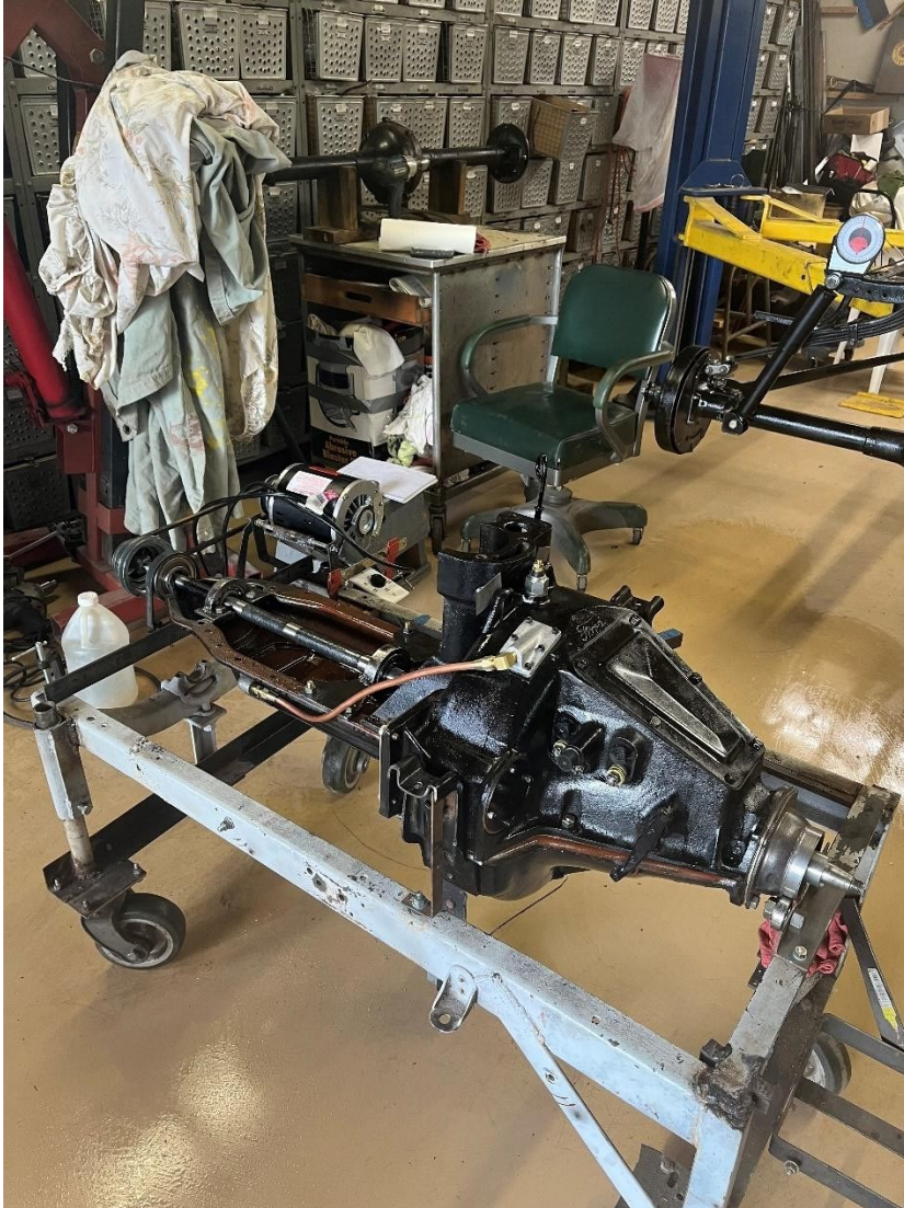
The mini dyno shown from the left side. Note the bearing at the rear which, with another bearing at the front, allows free rotation of the pan/hogshead/flywheel system.
