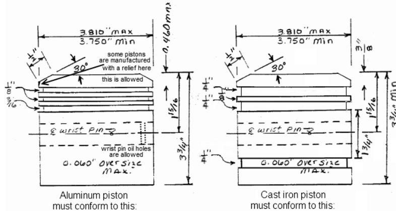
2.5.9.4. Drilling oil holes into wrist pin boss allowed. See above drawing.
