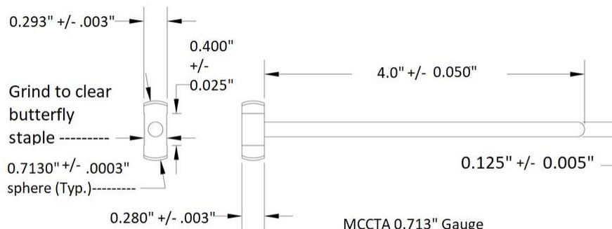
2.8.1.3.1. Also assure that the association's W-gauge does not engage the gauge handle when inserted through the choke throat, past the venturi, and into manifold side throat.
